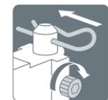
Reverse-thread screws and safety pin prevent damage or injury due to the speaker accidentally falling during installation.
