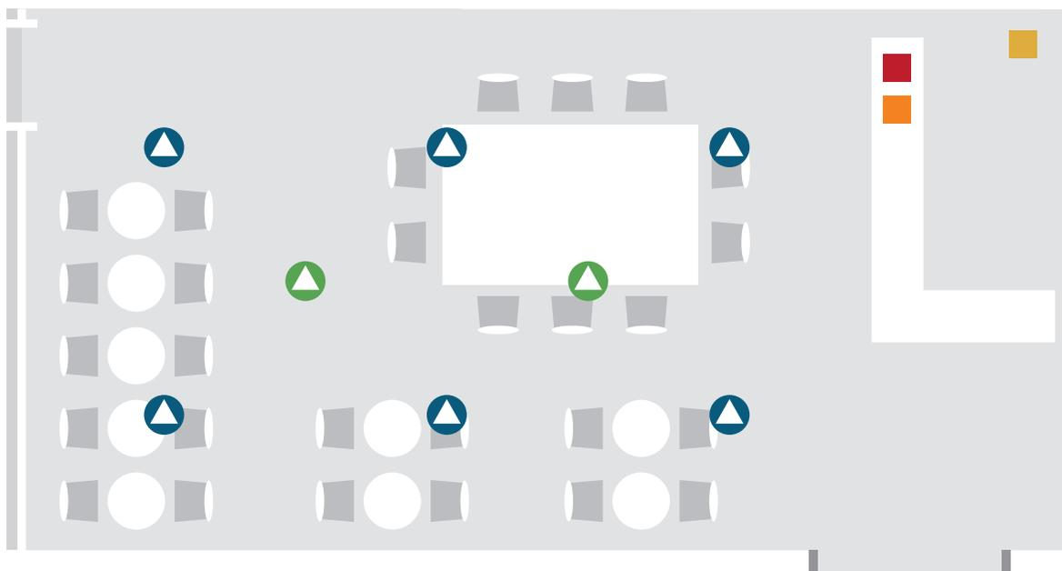
With VXC2F speakers and a mixer amplifier MA2030a, it is possible to create a streamlined, high-performance system that allows microphone use while background music is being played. Add a power amplifier PA2030a and a ceiling subwoofer VXC8S to create enriched ambient.
